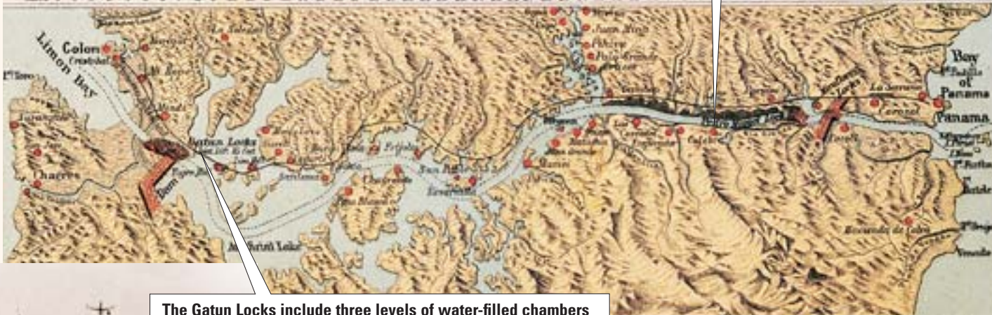
The Gatun Locks include three levels of water-filled chambers that raise or lower ships 85 feet. Electric locomotives called mules help guide ships through the locks.
